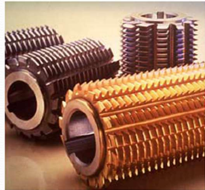
Figure 9. Typical carbide cutting tools brazed to metal in a brazing furnace. (Photo courtesy of Handy & Harman)
